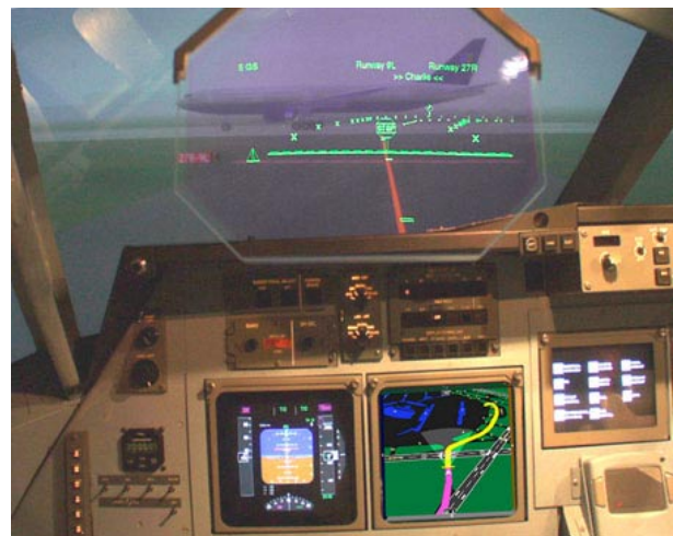
Figure 7. Taxiway Navigation And Situation Awareness System (T-NASA) (Source [32])
